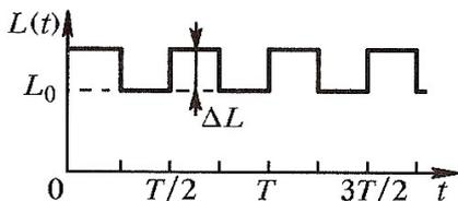
$$\Delta W = W_2 - W_1 = \frac{\Phi^2}{2} \frac{\Delta L}{L(L + \Delta L)} \approx \frac{\Phi^2 \Delta L}{2L^2}$$
